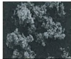
Microcapsules obtained by use of a Type-3 of particles
